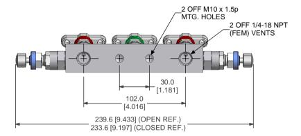
5 VALVE MANIFOLD DIRECT MTG INLETS: 1/2-14 NPT (FEM) VENTS: 1/4-18 NPT (FEM) MATERIAL OF CONSTRUCTION: SEE 'H-SERIES MATERIAL SPEC'.
